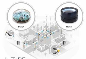
Smart street lighting based on massive IoT RF mesh communication providing the city an infrastructure for various other IoT sensor and thus promoting other smart city solutions.
