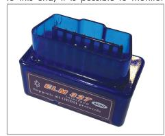
Snap4City Apps may have OBD2 module to access at the Vehicle data. The Mobile App module supports the users in (i) getting connected with the Dongle as Bluetooth device, (ii) observing the value and changes of all variables, (iii) the selection of a number of variables to create a separate view, (iv) the activation of real time save/upload of selected variables on the cloud of Snap4City services for their further reuse, Data Analytics and visualization, real time and historical.
