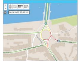
and in the high speed highways Fi-Pi-Li. The computation and dashboard show the city traffic in all primary and secondary street segments of the city representing the flow with a color coding, for each segment of 20mt. On the other hand, the traffic density is computed as a floating point data for each segment that can be profitably used for the above mentioned algorithms.
