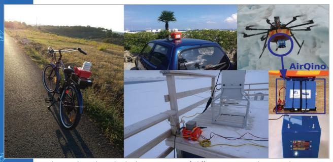
The AIRQino boards deploys a variety of different sensing elements that monitor different pollutants. These elements are based on different technologies. The gases monitored by AIRQino sensor board include also reactive gases, the air-flow inside the waterproof box is designed to minimize the gas interference. A small brushless fan blow air out the box. This create a depression that attract air from the inlet window.
