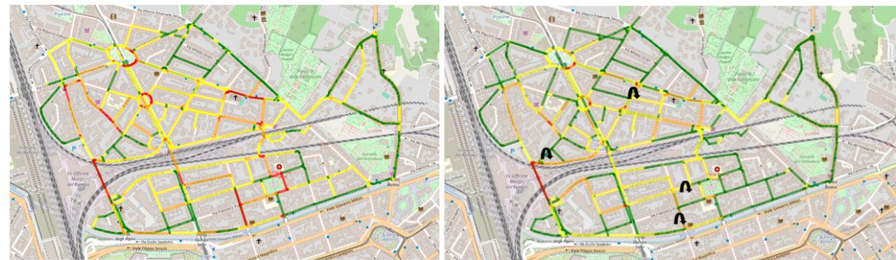
FIGURE 5 – Original road infrastructure as scenario 1 with ODM traffic at t1 = 2023-09-28T09:00:00. FIGURE 6 – Road infrastructure of scenario 1 with simulation based on traffic ODM at t1 ( morning ) after the changes (curved blue icons) suggested by Deep-RL-GNN by model_t1_time .
