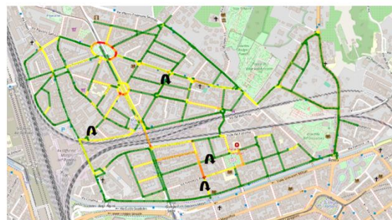
FIGURE 9 Road infrastructure of scenario 1 with simulation based on traffic ODM at t 2 (evening) after the changes (curved blue icons) suggested by Deep-RL-GNN by model_t1_time .
