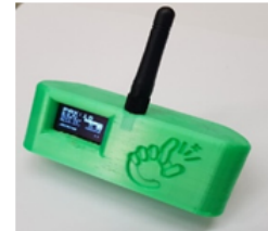
Figure 12: A mobile PAX counter based on ESP32.
