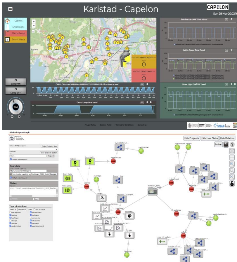
Figure 13: Example of a Dashboard and its graphical representation of the relationships among widgets, devices, Entity Instances and Entity Messages, etc. The tool on the right side is called LOG, LOGraph, Linked Open Graph and it is accessible from the dialog of Dashboard manager (not all Snap4City platform are provided with the LOGraph, it is optional and can be installed in a second phase).
