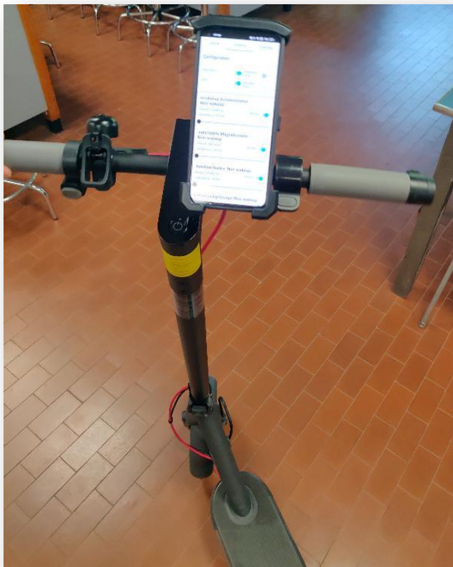
Smartphone-based measurement nodes (GNSS, IMU sensors)
