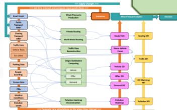
Figure 1: Conceptual Flow Diagram for a What-If analysis platform for mobility and transport with data, processes, simulations, outputs, and KPI.
